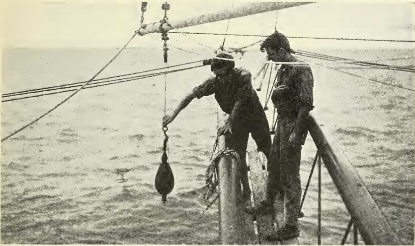
Fig. 12. The sounding weight and tube ready to go down.
